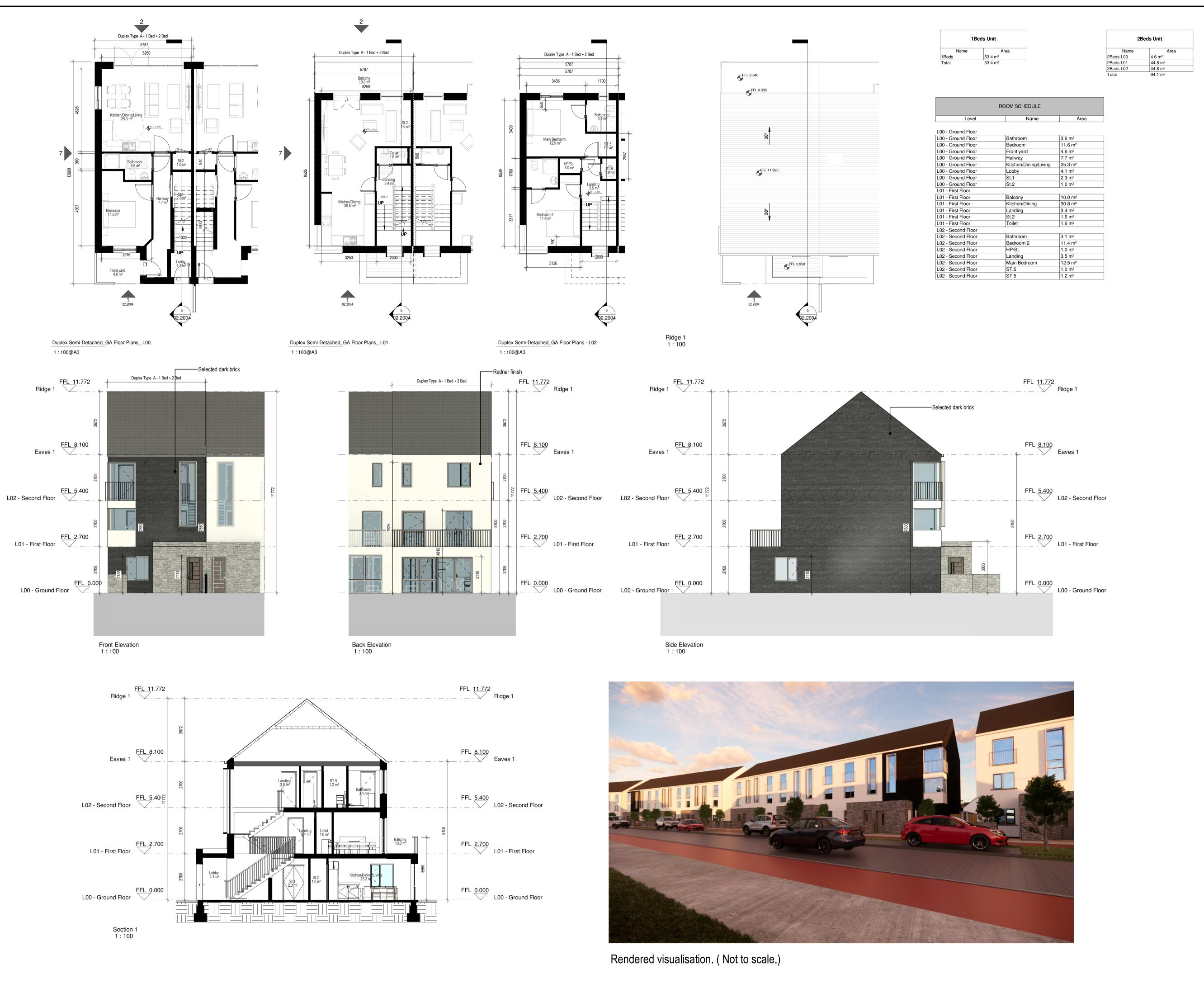
Selected clay bricks to varying colours as defined in the different character areas as indicated, painted nap sand cement render, expressed plaster bands around external opes / lintels. Concrete or metal cills, lintels or cappings as indicated on
